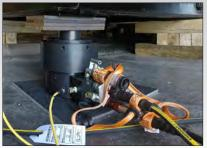
Custom doubleacting lock-nut cylinders with internal stroke sensors and an integrated load holding valve for lifting nuclear components.
