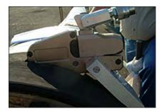
Custom hydraulic torque wrenches with reaction paddles for use with a flexible flowline.
