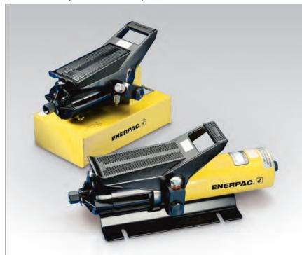
PA **Series Reservoir Capacity:** 36-80 in<sup>3</sup> Flow at Rated Pressure: 8 in<sup>3</sup>/min. Maximum Operating Pressure: 10,000 psi
