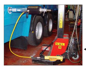
An RACH-306, powered by a P-392 hand pump, is used to extract corroded carriage pins from refuse collection vehicles.
