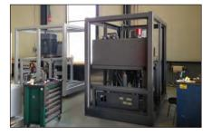
**HYDRAULIC POWER UNITS** Enerpac designs, assembles and tests small to large hydraulic power units in-house. Power units range from 0.5 to 300 hp and are tested with the system they are intended to operate.
