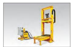
100-Ton Press for Assembly of Spring-Loaded Cylinders
