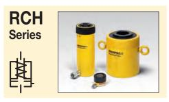
Capacity: 12-100 tons Stroke: .31-6.13 inches Center Hole Diameter: .68-3.11 inches Maximum Operating Pressure: 10,000 psi
