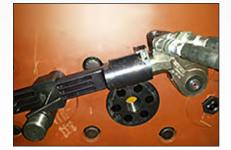
Custom hydraulic torque wrench for a fracking pump.
